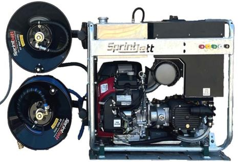
The Softwash Systems Trolley connects to your existing pressure cleaner, by connecting your pressure cleaning hose to the inlet of the portable softwash trolley
